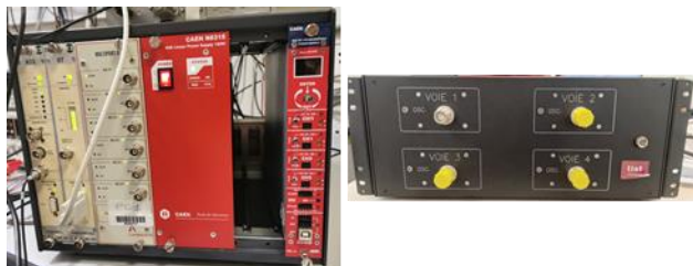
Fig. 1. View of the 7820-7821 modules from Canberra (left) and the new digital readout electronics developed at CEA List (right).
