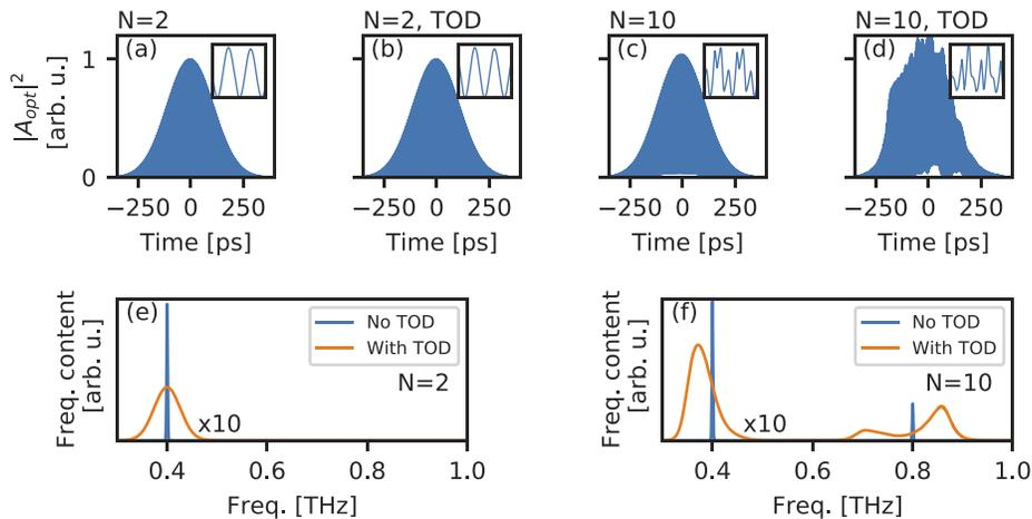
**Fig. 2.** Comparison of the total pulse train envelope (a-d) and frequency content (e-f) for a pulse train of  $N=2$  and  $N=10$  pulses and drive pulses with and without TOD. In this specific example the THz frequency is centered at 400 GHz with pulses (GDD= $2.3 \text{ ps}^2$ , TOD= $-0.0044 \text{ ps}^3$ ) delayed by  $\Delta t=5.78 \text{ ps}$ . Insets in panel (a-d) show a zoom from 150–156 ps which captures the temporal interferences responsible for the difference frequency content.
