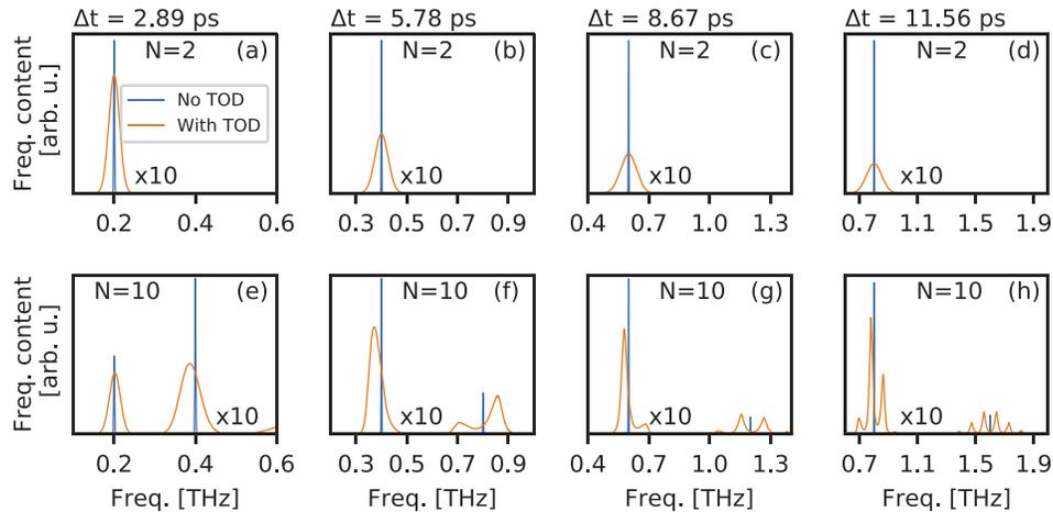
**Fig. 3.** Comparison of the total pulse train difference frequency content at many time delays. We show the same permutations of no TOD (blue) and a TOD of  $-0.0044 \text{ ps}^3$  (orange),  $N=2$  pulses (a)–(d) and a pulse train ( $N=10$ ) (e)–(h), at the four different delays  $\Delta t=2.89$ , 5.78, 8.67, 11.56 ps necessary to produce frequency content centered on 200, 400, 600, and 800 GHz respectively. Panels (b) and (f) are a duplication of Figs. 2(e) and 2(f).
