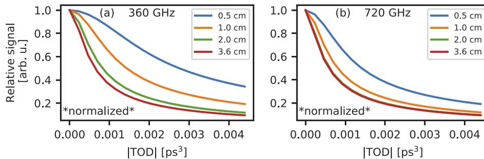
**Fig. 8.** The relative decrease in THz generation efficiency due to TOD for different frequencies and lengths with the ANGUS pump parameters in PPLN. In all cases as the TOD increases the efficiency drops monotonically relative to the case with zero TOD. Calculations are made with the FFT+analytic method using Eq. (1) and therefore do not take in to account nonlinear cascading. Shown are results for 360 GHz (a) and 720 GHz (b) at lengths of 0.5, 1.0, 2.0, and 3.6 cm.
