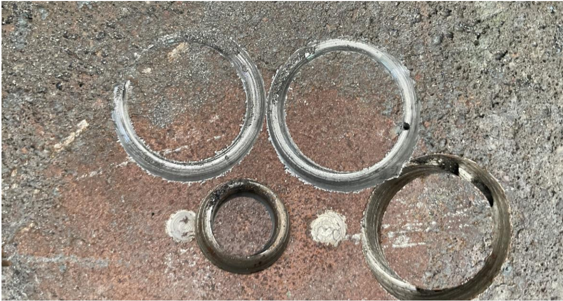
Figure 14: View of VF-08 metallic block after 3 core boring tests with \varnothing 25 mm tool and one (lower left) with \varnothing 15 mm tool
