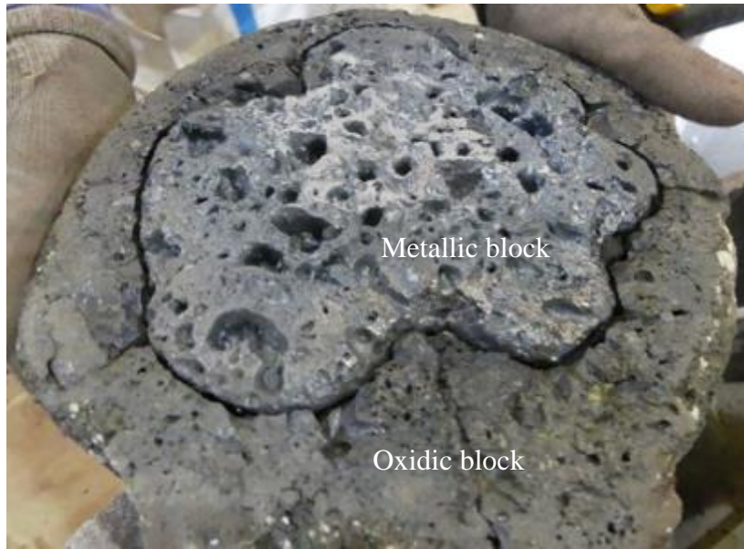
Figure 2: VF-U3 Ex-vessel fuel debris prototype: upside-down view of lower part (approximate diameter: 25-26 cm)
