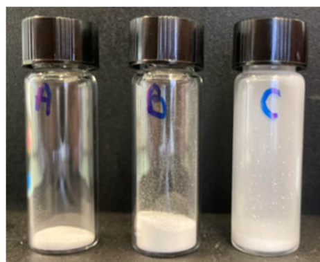
Fig. 6 Pictures of CB, SiO 2 CC and Celite® CC for the coating of Xantphos (targeted coating charge of 5% w/w for Silica and Celite® and 6.31% w/w for CB)
