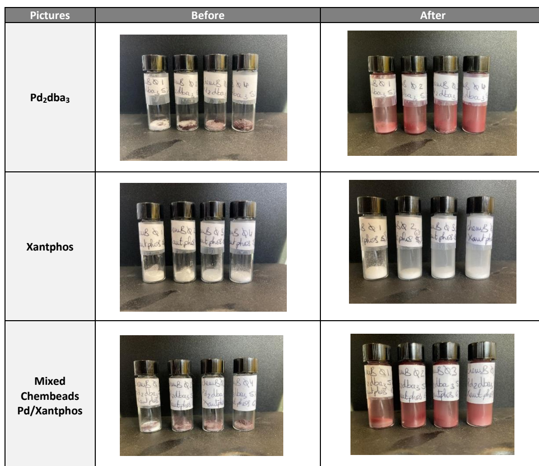
Figure S1: Preparation of Chembeads of four different sizes before and after mixing
