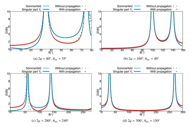
Fig. 9: Diffraction coefficient computed with the spectral functions and with the Sommerfeld method, in the case of Neumann boundary conditions.
