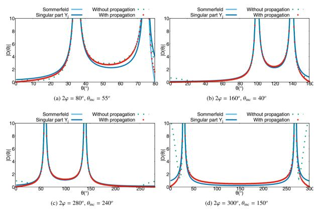
Fig. 8: Diffraction coefficient computed with the spectral functions and with the Sommerfeld method, in the case of Dirichlet boundary conditions.
