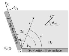
Fig. 1: The wedge of angle  $2\varphi$  whose faces are stress-free is illuminated by a plane wave of wave vector  $\mathbf{k}^{\text{inc.}}$ .
