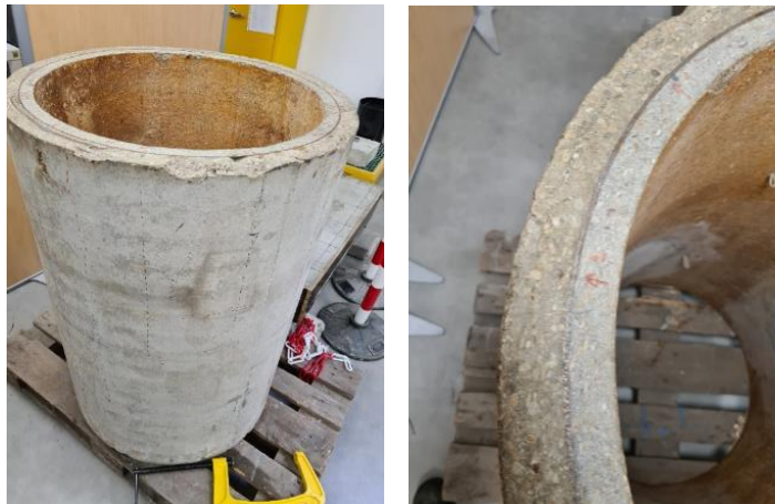
Figure 1: Pictures of a sample of a concrete/steel/concrete pipe
