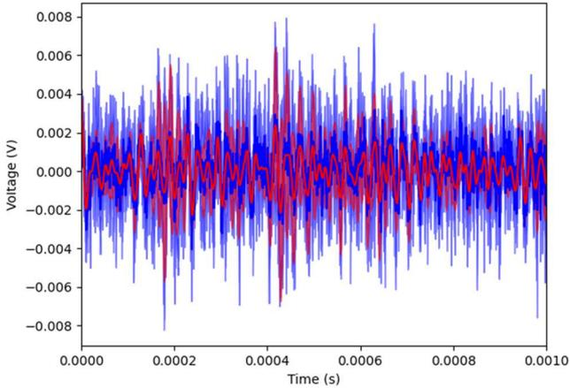
Figure 4: Residual signals using the data acquired in the static case as a reference. Lines correspond to the mean signal over different acquisitions, shaded areas correspond to 3 standard deviations around the mean value. Blue: raw signal. Red: band-pass filtered signal.
