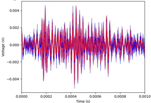
Figure 5: Residual average signals using the data acquired in the static case as a reference averaging each acquisition over 10 consecutive samples. Lines correspond to the mean signal over different acquisitions, shaded areas correspond to 3 standard deviations around the mean value. Blue: raw signal. Red: band-pass filtered signal.
