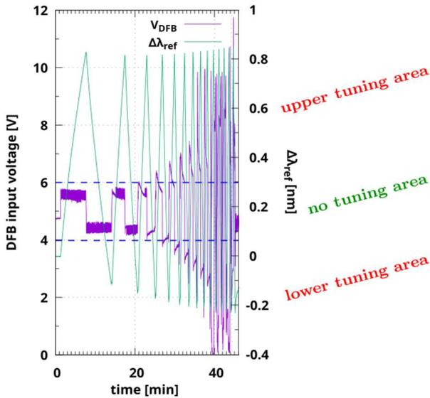
Figure 2: Evolution during the four points bending test of the DFB laser diode control DC input voltage  $V_{DFB}$  and the wavelength shift  $\Delta\lambda_{ref}$  of a control FBG transducer glued on the flat composite sample.
