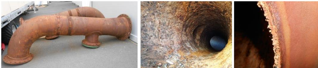
**Figure 6:** Pictures of a steel pipe affected by corrosion
