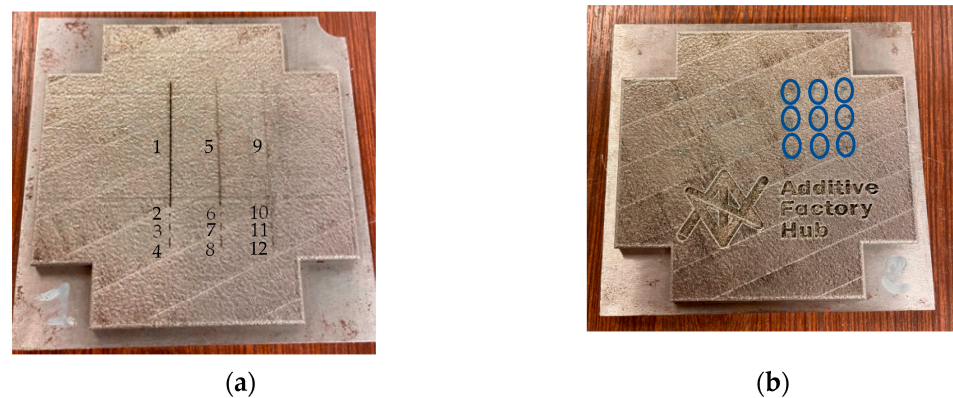
Figure 2. Designation of stainless steel 316 L mock-ups (a) with artificial defect (b) with nine cylindrical defects (encircled in blue) and letters printed during part manufacturing.
