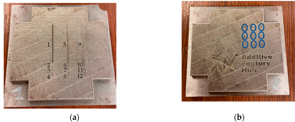
Figure 2. Designation of stainless steel 316 L mock-ups (a) with artificial defect (b) with nine cylindrical defects (encircled in blue) and letters printed during part manufacturing.
