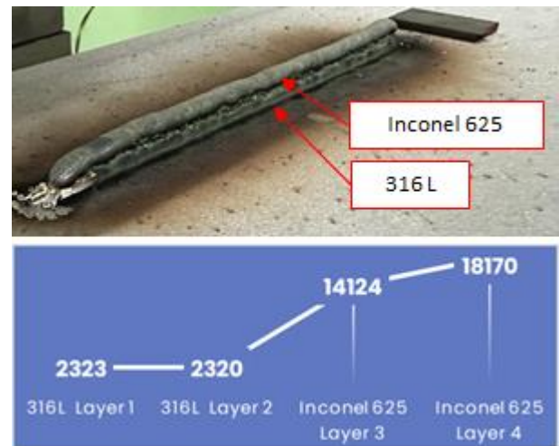
Figure 4: Picture of a two wires coupon (top) and the associated variation in the count of the Nickel ray of fluorescence (bottom).
