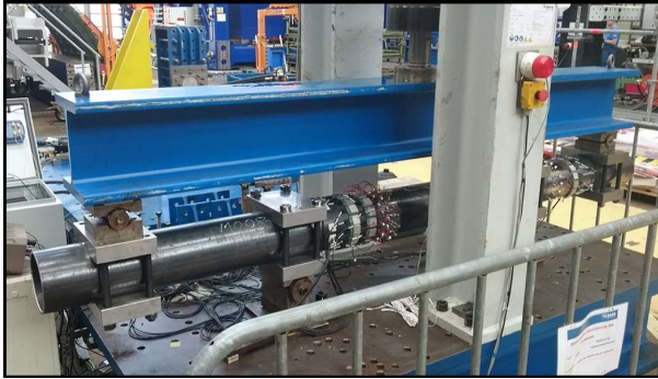
Test stand of 4-point bending tests at IMA Dresden GmbH within the project QuantSHM (funding code 100207022) which was funded by the federal state of Saxony via the Sächsische Aufbaubank. (Image provided by Fraunhofer IKTS, a partner in the GW4SHM project.)
