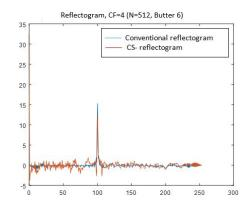
Fig. 9. Reflectogram generated with the conventional reflectometry architecture at 200 MHz (blue curve), reflectogram generated with the reflectometry architecture based on CS at 50 MHz (N=512 samples, CF=4, Butterworth filter of order 6 and  $f_c$ =25 MHz).
