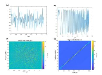
Fig. 3. (a) The time representation of the classical OMTDR signal. (b) the time-frequency representation of the classical OMTDR signal. (c) the time representation of the OMTDR signal in chirp form (d) the time frequency representation of the OMTDR signal in chirp form.
