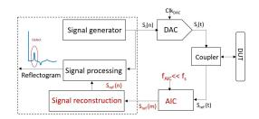
Fig. 2. Schematic diagram of CS-based reflectometry architecture
