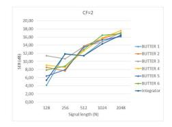
Fig. 5. Evaluation of the SER as a function of the number of signal points and the nature of the filter (cutoff frequency  $f_c$ =50 MHz for Butterworth filters) for a compression factor of 2.
