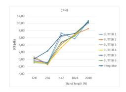
Fig. 7. Evaluation of the SER as a function of the number of signal points and the nature of the filter ( $f_c$ =12.5 MHz for Butterworth filters) for a compression factor of 8.
