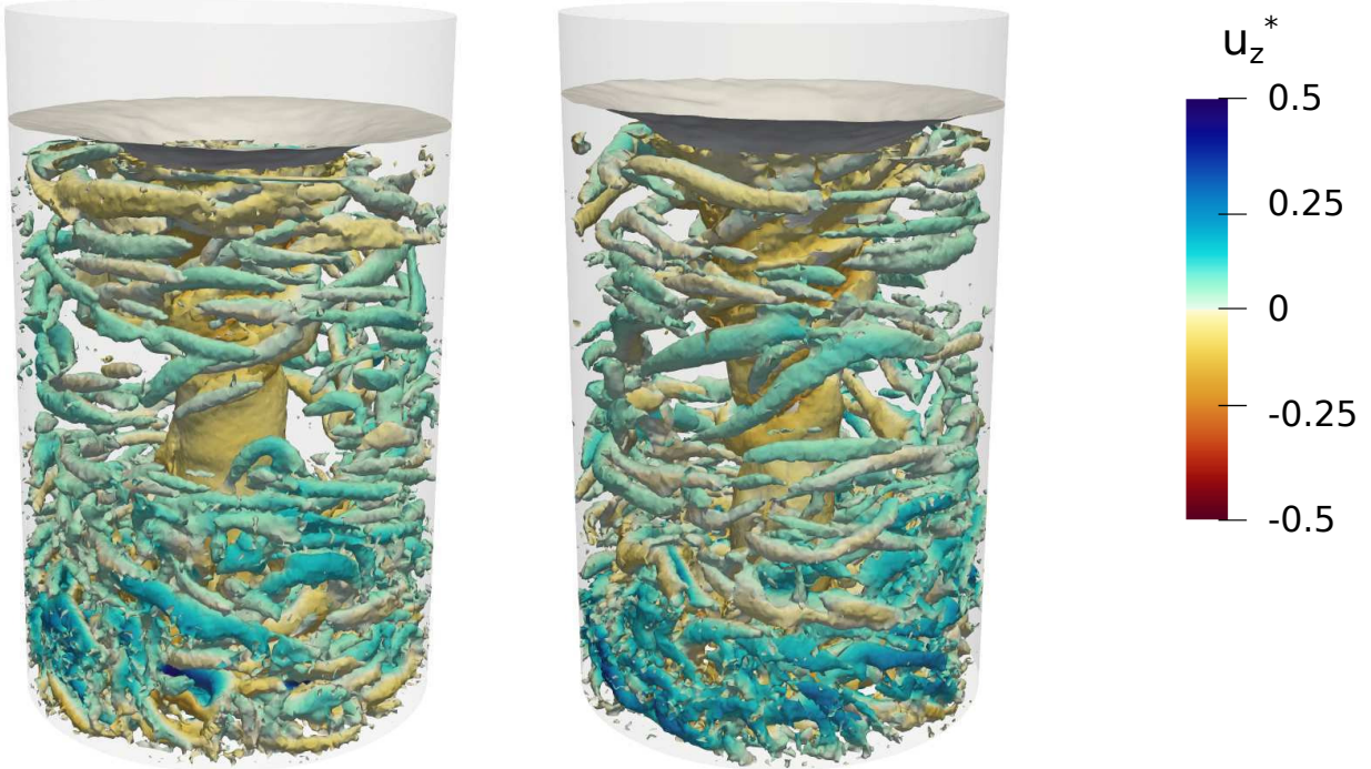
Figure 6: Instantaneous iso-surfaces of the Q-criterion colored by the vertical velocity component u_z^* at t^* = 118 . Left: Re_{s1} \approx 7 \times 10^4 , right: Re_{s2} \approx 8.6 \times 10^4 .
