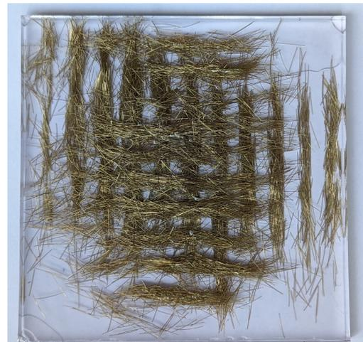
**Figure 5:** A cross-layered specimen showing the steel fibers in a cross-layered pattern
