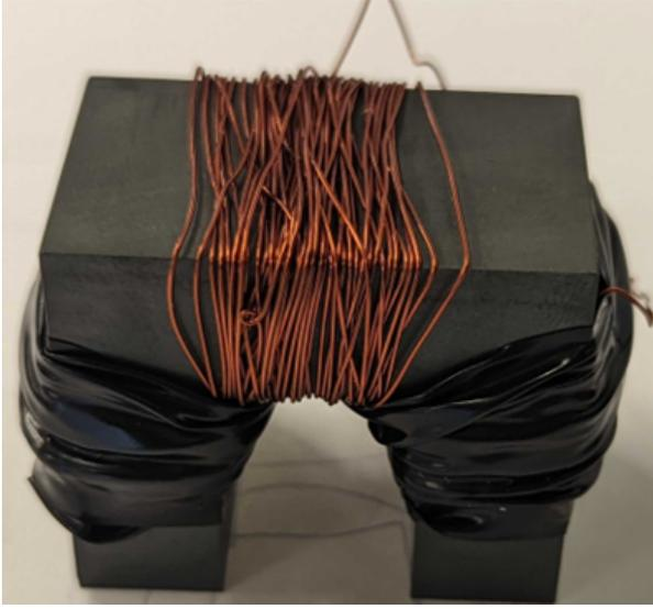
**Figure 7:** A magnetic sensor/inductor made with 150 turns of 0.5 mm magnetic wire wrapped around a U-shaped ferrite core.
