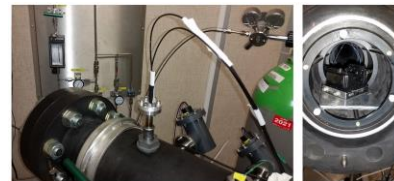
Fig. 5. View of the calibration experiment with the flame propagation tube (left), probe blocked inside the tube (right).
