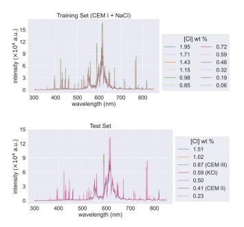
Fig. 4. Average spectra of the cement samples. Samples were fabricated using CEM I, with the addition of NaCl, unless otherwise stated.
