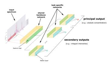
Fig. 2. The MT model is a hard parameter sharing structure, that is a common backbone network and several heads, connected to the shared feature map.
