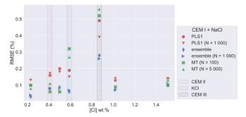
Fig. 7. Prediction uncertainties of the MT model on cement samples as a function of training set size.
