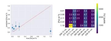
Fig. 8. Comparison of ground truth and predicted values on the Ti matrix, using a model trained on the Co matrix.
