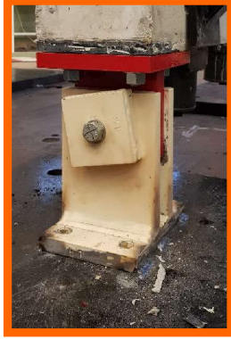
FIGURE 2: Details on the components realizing the boundary conditions with the Azalée shaking-table.
