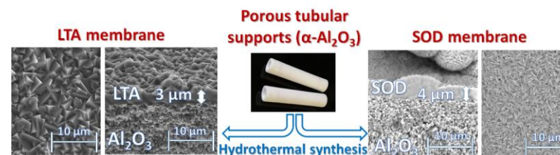
Figure 1. SEM micrographs of LTA and SOD zeolite membranes deposited on the inside of tubular alumina supports.
