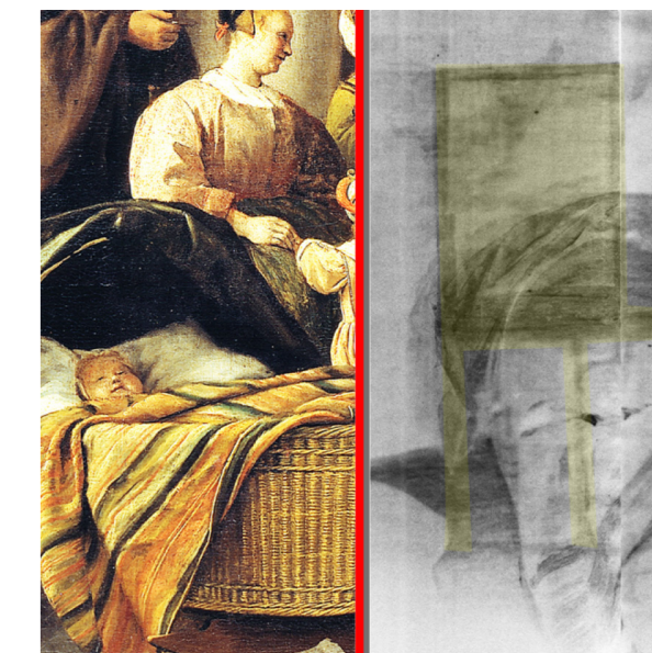
Neutron autoradiography of the 17th century Dutch painting ‘As the old ones sing, so the young ones pipe’ by Jan Steen, reveals it to be an adaptation of an originally very different composition. © Helmholtz-Zentrum-Berlin.
