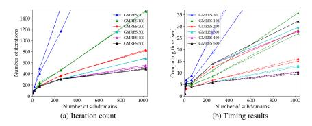
Fig. 5: Weak scaling results for the  $2 \times 2$  to  $32 \times 32$  square decompositions, using various GMRES restart parameters. Volume methods (solid lines) and substructured methods with (dashed lines) or without (dashdot lines) diagonal transfer are used.
