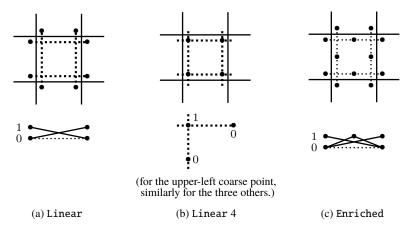
Fig. 6: Schematic view of substructed coarse space options, with coarse point positions (above) and coarse function sketch (below).
