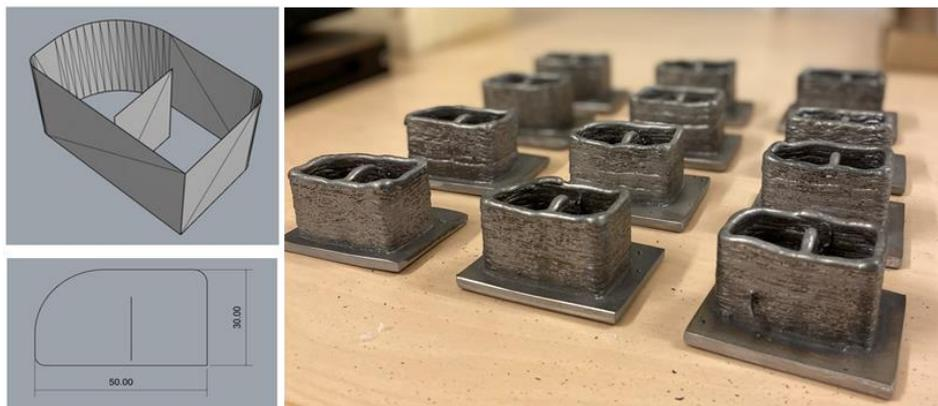
Figure 1. The nominal size of the coupons (left) and the all the manufactured coupons
