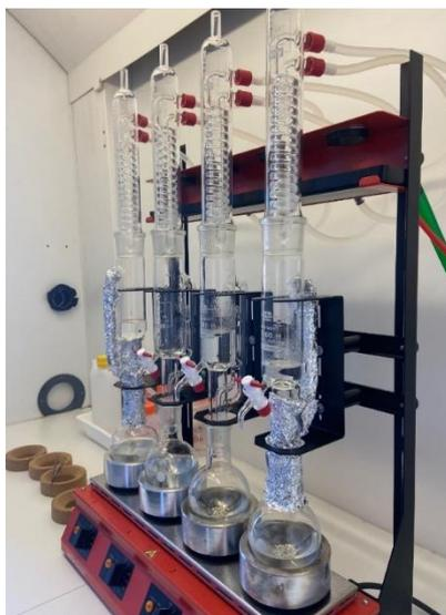
Figure 5 Multi-column Soxhlet extractor installation at laboratory
