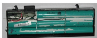
Notebook battery 8 cells in 18650 size 4s2p type assembly Max. open circuit voltage: 16,8 V
