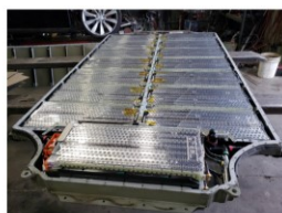
Tesla model S battery (2014) 8 256 cells in 18650 size 96s86p type assembly Max. open circuit voltage: 403,2 V
