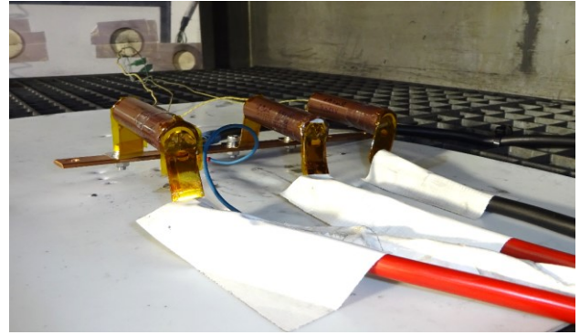
Fig. 8 Photograph of the experimental installation. Three cells in parallel in a test chamber before the experiment.
