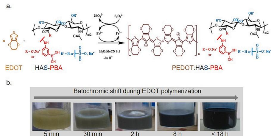
Fig. 3. Reaction scheme (a) and solution color change (b) during EDOT polymerization in the presence of HA derivatives.
