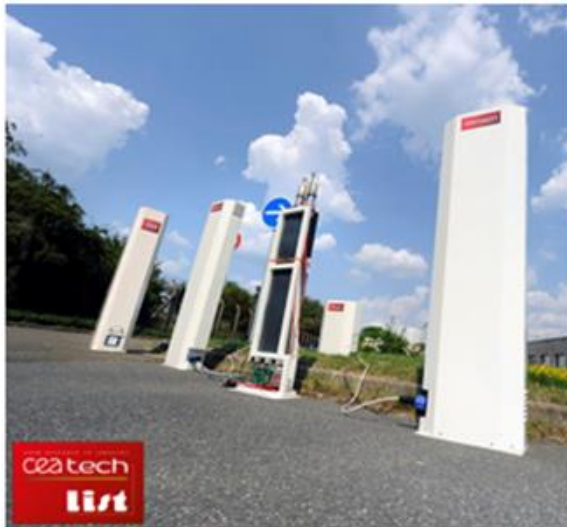
Example of plastic scintillator based RPM
