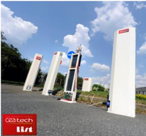
Example of plastic scintillator based RPM
