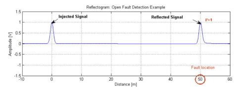
Figure 1: Reflectogram with and open circuit at the end of the cable [3].
