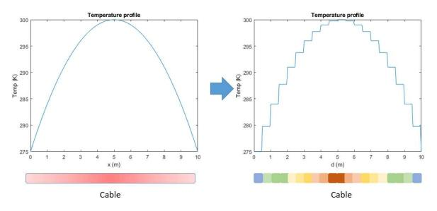
Figure 2: Presentation of the principle of the ABCD mesh.
