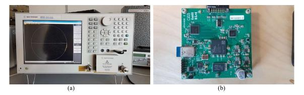
Figure 5: TDR measurement tools: (a) a Vector Network Analyser (VNA), (b) CEA TDR sensor.
