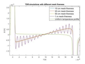
Figure 3: TDR response based on ABCD mesh modelling.
