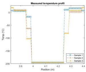
Figure 11: Temperature profile along the cable under test.
