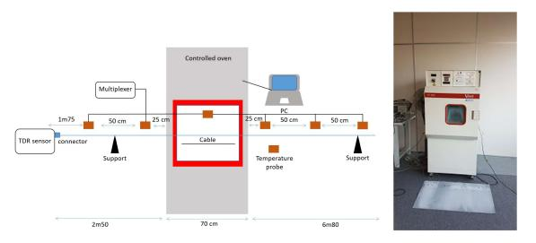
Figure 8 presents the schematic of the experiment and the photography of the Vötsch VT7010 controlled oven used for the experiment.
