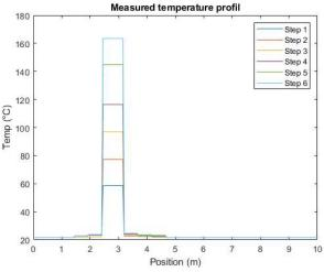
Figure 13: Temperature profile along the cable under test.
