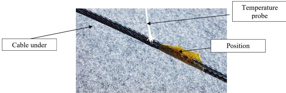
Figure 6: Probe set up.
