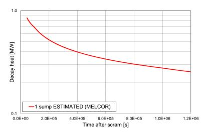
Figure 3 Decay heat of debris in a single sump based on SNL calculations
