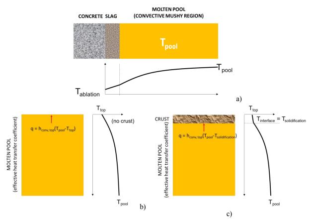
Figure 5 Schematic view of the heat transfer network employed in the ASTEC/MEDICIS code and the COCOSYS/AC<sup>2</sup> code. a) heat balance on the concrete side, b) and c) the two different states on the top surface
