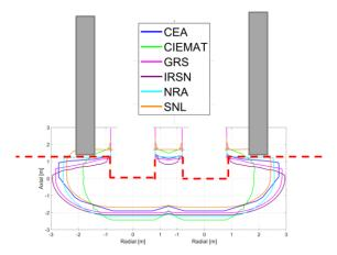
Figure 12 Predicted erosion end configuration in comparison with the pedestal walls
