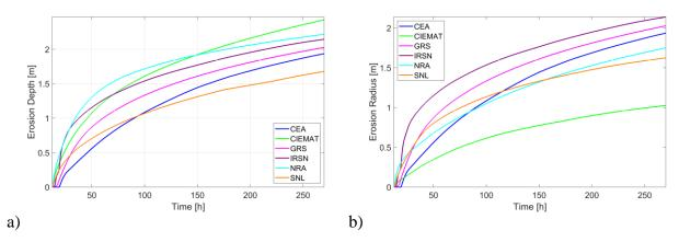
Figure 9 Maximum concrete erosion a) vertically and b) radially
