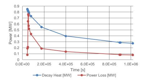
Figure 4 Decay heat and top boundary power loss imposed in the simulation
