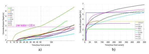
Figure 1 BSAF phase 2 results of the MCCI vertical erosion for Unit 1 [[2]]
