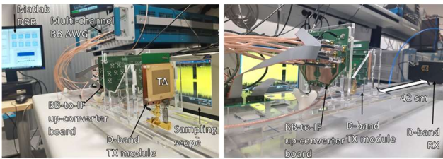
Fig. 7. Point-to-point D-band link set-up.
