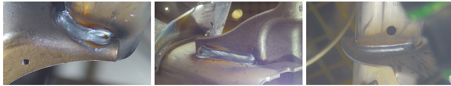
Fig. 5. Welds C10, C20 and C34 of a rear axles production line. (from left to right)
