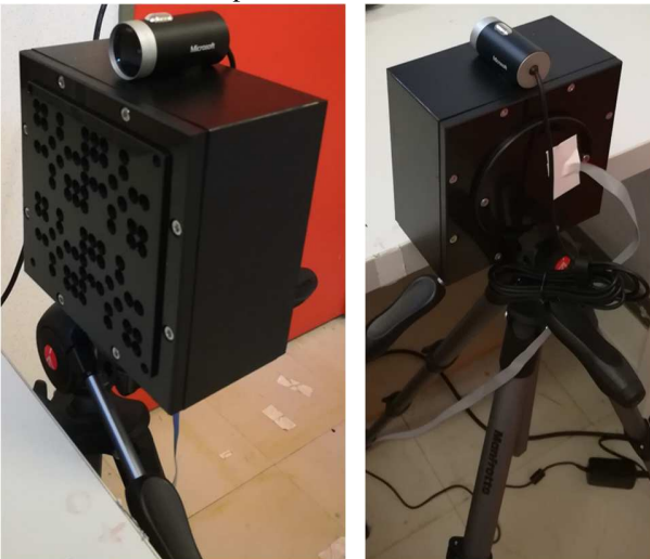
Fig. 20. Prototype of the gamma-neutron imager based on pixelated plastic scintillator and coded aperture.
