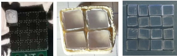
Fig. 2: Pixelated PS. Left: 1×1 PS #2.1. Middle: 2×2 PS #2.2. Right: 4×4 PS #2.3.
