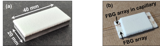
Fig. 1. (a) APS target for OFS embedding. (b) Embedded sensors in cordierite after the first thermal annealing.
