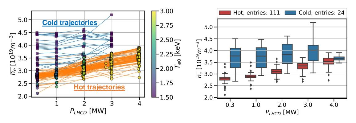
Hot trajectories fix an **upper boundary for density** at given LHCD power
