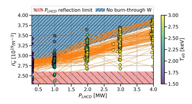
Upper density limit (No burnthrough W) is taken as the 80<sup>th</sup> percentile of hot pulses trajectories (conservative)
