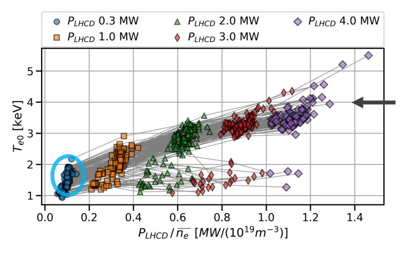
Goal of heating phase: **burn-through tungsten** and reach **hot branch**  $(T_{e0} > 3 \text{ keV})$
