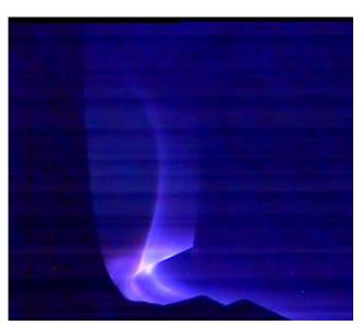
**WEST** is a device specialized for long pulse operation in a tungsten environment. Testbed for ITER divertor technology (actively cooled tungsten mono-blocks)
