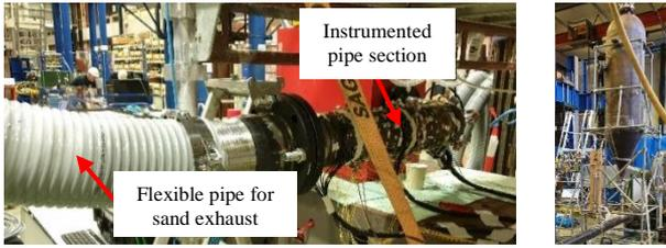
Figure 2: The studied structure is mounted to the erosion loop (left) and the sand vessel (right).
