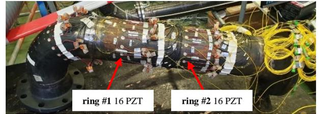
Figure 1: The studied structure instrumented with two rings of PZTs.
