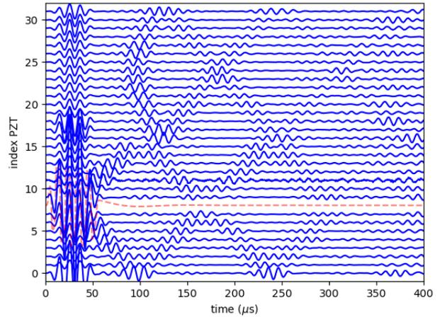
Figure 4: Signals for an emission with PZT #8 before the erosion loop starts.
