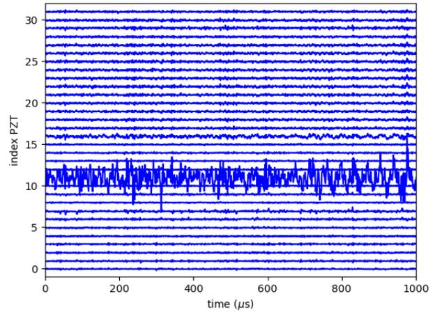
Figure 8: Small portion of the ambient noise measured by all the sensors when the erosion loop is out of operation.
