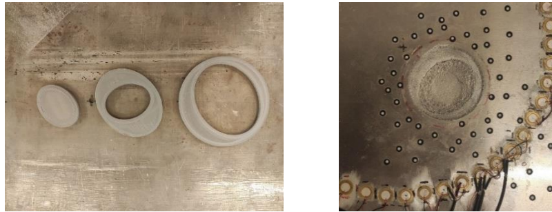
Figure 3: Elliptic masks and third defect created by electrolysis.
