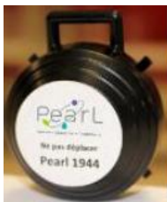
Based on solid-state nuclear track detector (SSNTD)
