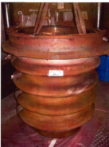
Fig. 9. A bellows tested on Superphenix heat exchanger.
