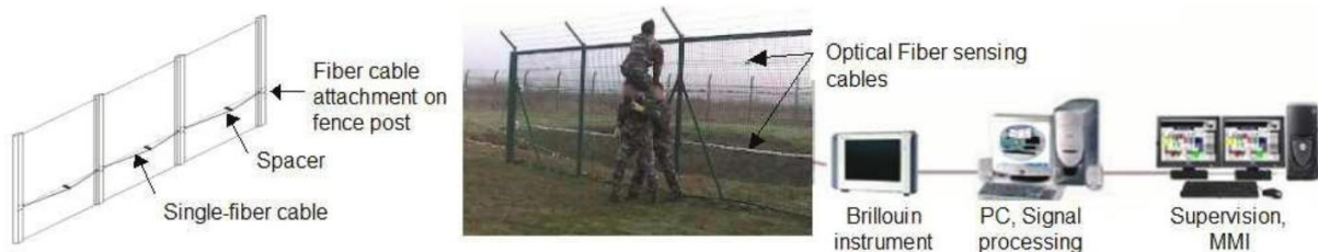
Figure 4. Cable deployment and SMARTFENCE system, when commandos climb over the fence (credit CEA).
