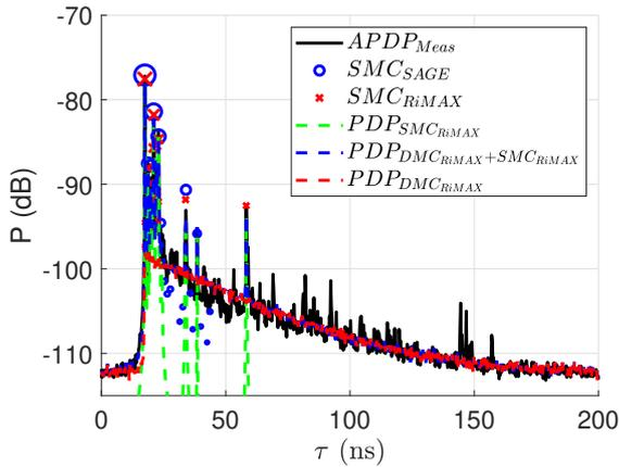
Fig. 3: Average Power Delay Profile (APDP) at P5 with RiMAX/SAGE estimates.
