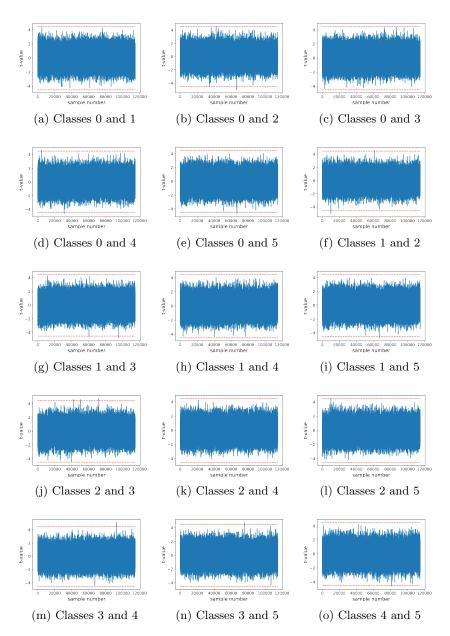
Fig. 6: Welch t-test results between each classes using 10,000 traces of randomly sampled inputs within the classe. The trace correspond to the FHT with the counter-measure. -4,5 and 4,5 are plotted with dashed red lines.
