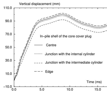
Fig. 14: Vertical displacement of the CCP in-pile shell
