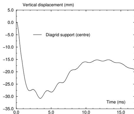
Fig. 13: Vertical displacement of the diagrid support
