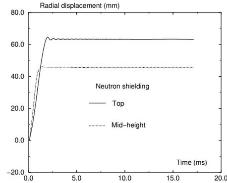
Fig. 16: Radial displacement of the neutron shielding
