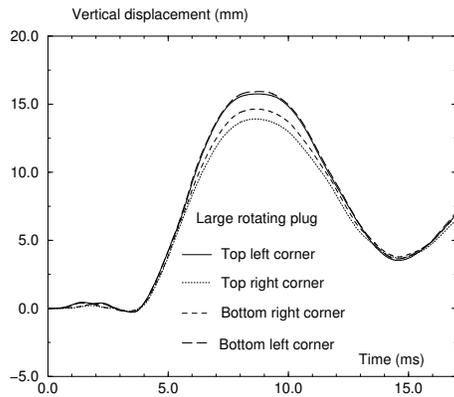
Fig. 11: Vertical displacement of the large rotating plug
