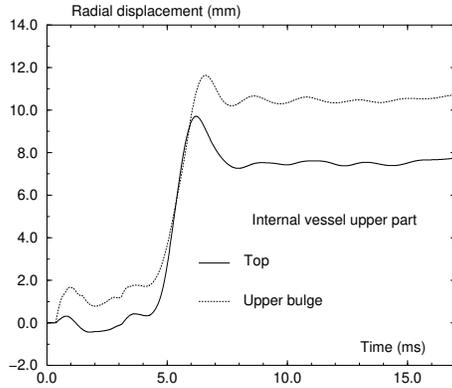
Fig. 19: Radial displacement of internal vessel upper part
