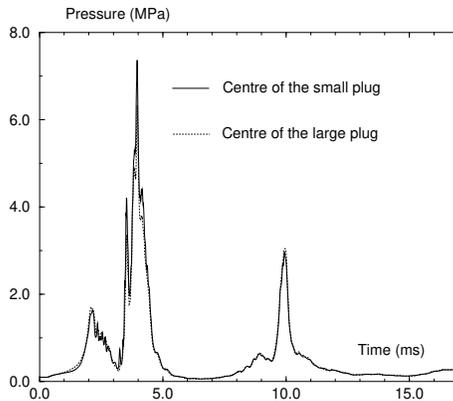
Fig. 21: Pressure under the two rotating plugs
