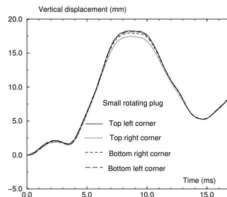
Fig. 10: Vertical displacement of the small rotating plug
