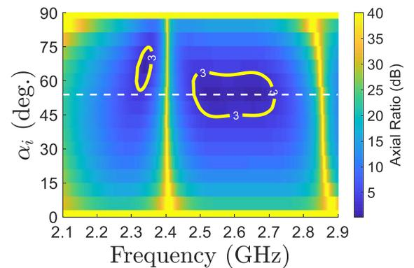
Fig. 4. Measured Axial Ratio as a function of both frequency and slant angle  $\alpha_i$  with a  $6^\circ$  step (the yellow contours indicate the regions where the axial ratio is lower than 3 dB and the dashed white line highlights the axial ratio in function of frequency at a fixed slant angle  $\alpha_i = 54^\circ$ )
