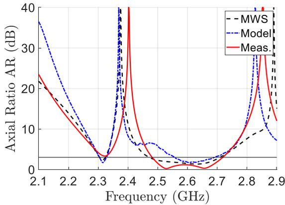
Fig. 5. Axial Ratio, as function of frequency at fixed  $\alpha_i = 54^\circ$ , obtained from: full-wave electromagnetic simulation (CST MWS, black dashed curve), the electromagnetic model of Section II (blue dotted curve) and direct measurements (red solid curve).
