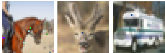
Fig. 1: CIFAR10 images correctly predicted ( horse, deer, truck ) by a ResNet model. Left: OPA selects a set of 10 sensitive pixels. These pixels are exhaustively tested with bit-flip perturbation. Middle and Right: a successful one bit-flip attack on a single pixel that respectively fools the model to cat and ship .
