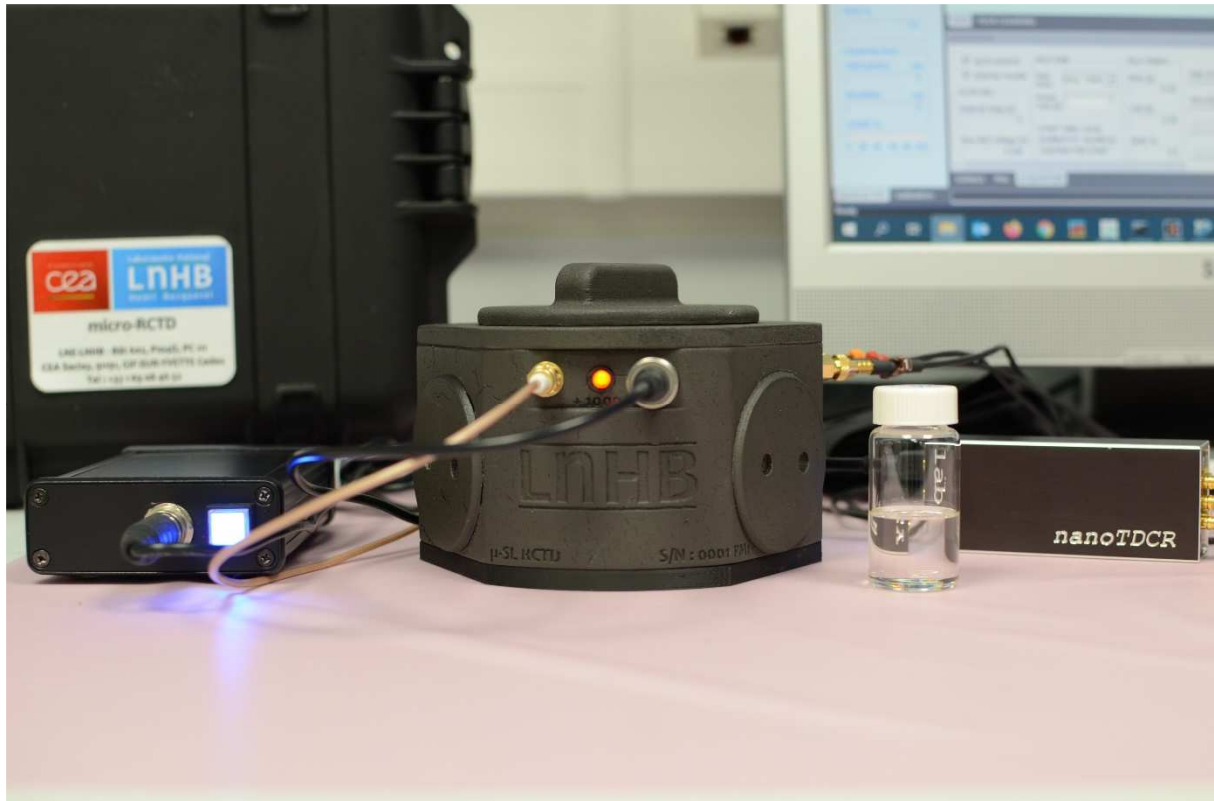
Figure 5: The \mu TDCR setup at LNHB with (from right to left) the nanoTDCR module, an LS sample, the 3D-printed detector housing containing the optical chamber and PMTs, a HV power supply and a transport case in the background.
