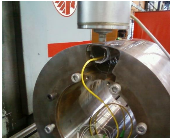
FIG. 17 View of the calibration experiment at AM R&D involving a load sensor.
